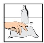
Clean the surface using an appropriate cleaner and wait until the surface is completely dried.
