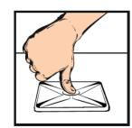
Put the base on the cleaned surface, pressing down with the finger for several seconds.
